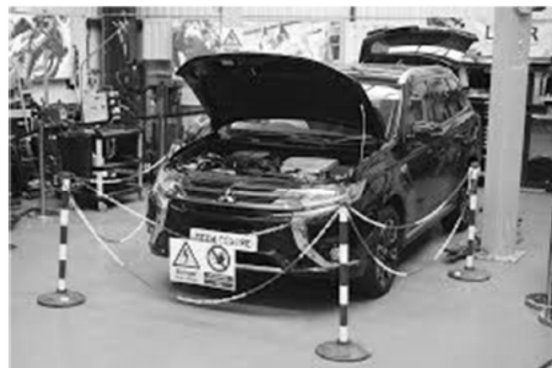
Figure 3. Example of a HVEVs maintenance area that is isolated and demarcated
