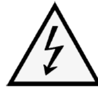
Figure 1. Marking of HV equipment
