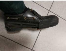
Safety shoe caps are not sufficient for high-risk jobs like maintenance not even for temporary works; they leave most of the body-part unprotected. they are usually provided to external contractors as a "shortcut" when they latter have not brought their own PPE.
