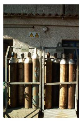
Good practice: metal cages are used in this metalworking workshop to store oxygen bottles; the pressurized bottles (right) are kept separate from the "empty" (to be refilled) ones (left); relevant signage is mounted on the wall
