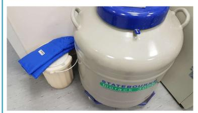
Cryogenic fluid in a lab; special precautions should be taken; cryogenic fluids should be stored in a separate area properly demarcated and not in plain access for everyone
