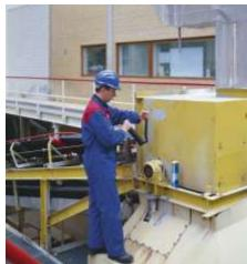
**Malpractice:** Use of unsuitable lubrication. Quantities of lubrication not optimized. Poor lubrication can impact energy consumption as well as cause failures (increase risk of contamination and spare part consumption).
