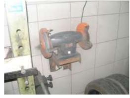
Grinding wheels with the protective covers removed.
