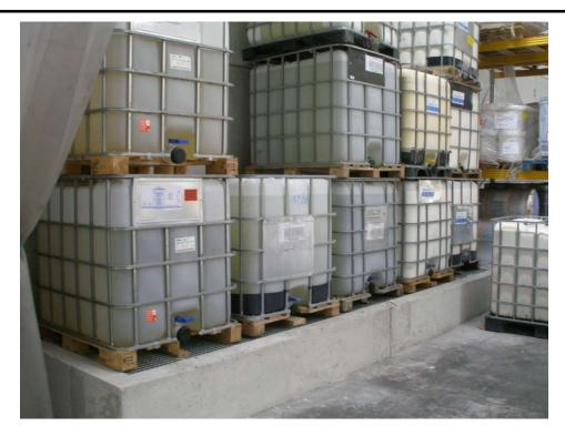
Secondary containment in a warehouse which is not correctly implemented; the dike capacity is sufficient but the storage height is too high thus creating a spill risk during the transportation of the IBC containers
